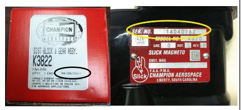
Figure 1. Replacement Kit Box Label Date Code Figure 2. Magneto ID Label Date Code
