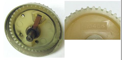
Figure 3. Affected K3008 Distributor Figure 4. K3008 Distributor Gear **Gear With Copper Electrode**
